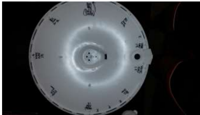
Black lines along edges are places material should be removed. Note other markings for LED placement. You'll need to remove or drill holes for the Nav lights and RCS thrusters as marked as well.
