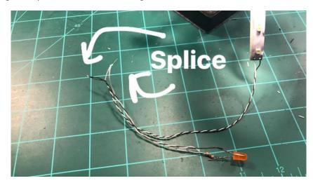
A "pigtail" is similar to a splice except, in this case, we'll twist multiple (common positive, for example) wires together from several LED's with one additional wire attached to go back to the terminal. That way, instead of trying to fit 10 wires into one terminal, you can simply have one. You will likely want to cover up the splice point of the pigtail with electrical tape or shrink tubing to avoid any possibility of crossing other wires and causing a short.
