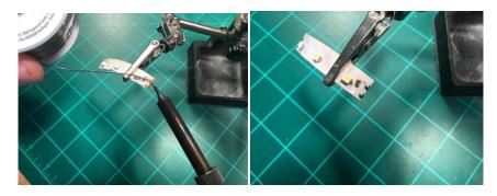
Notice that at the connection points, there is a positive side and a negative side. This is where we will add some solder before attaching the wire. (called "tinning" the solder point) Again, touch the solder coil and soldering tip together to the copper solder points, not just the iron tip with solder on it. "Drag" the melting solder from the solder coil onto the copper pads. You should have a small bead of solder at the point when finished.
