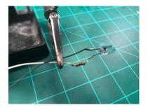
Next, repeat the same process with the wire by coiling about a cm of exposed (stripped) wire around the other end of the resistor and adding solder the same way. Then repeat this step for the negative wire and LED leg. (NOTE: you only need a resistor on one LED leg) Again, trim off any excess LED leg metal.
