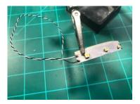
Next, strip off only about a half a millimeter of wire to attach to the points. Simply touch the iron tip to the solder point to re-melt the solder and slip the exposed wire into it and remove the iron, holding the wire still a second or two until the solder hardens. Repeat the process for both positive and negative contact points. That's it! It's wired!
