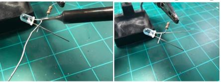
Next, slide the coiled resistor up the LED leg a bit and apply the solder by touching the iron and the tip of the solder coil to the wrapped resistor. For most LED's, you should keep your soldering iron from 335°C to 400°C. Leave just enough solder to secure the two wire leads together. Then trim the excess wire from the LED leg and the resistor leg, making sure not to cut into the solder itself and separate the two again.
